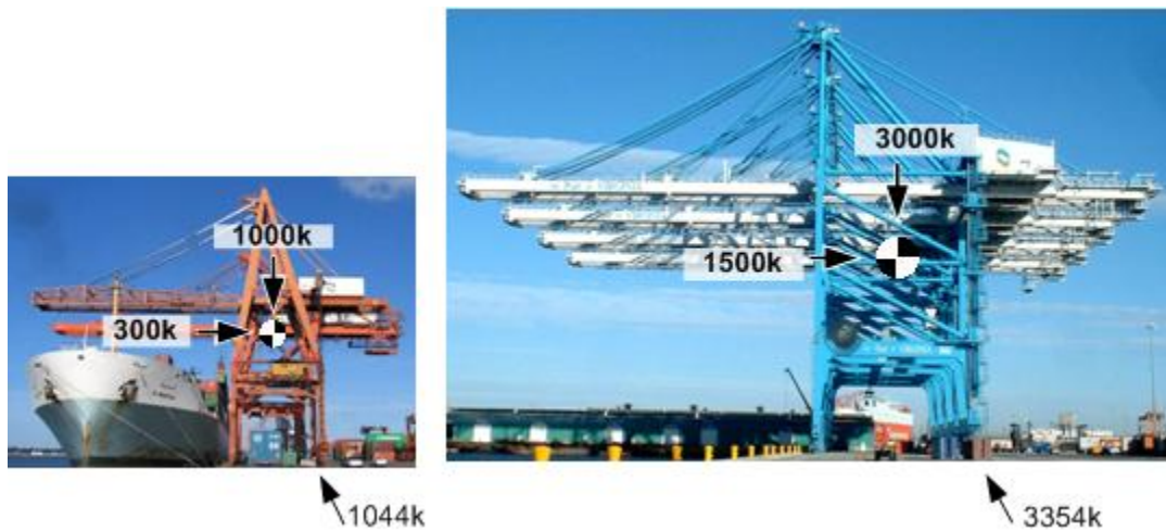
Figure 1. Small crane and jumbo crane tipping forces
